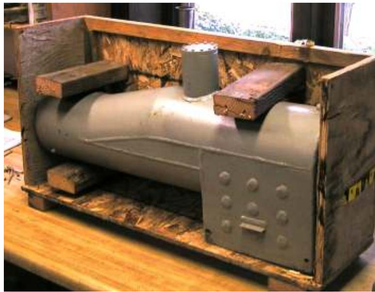
Kenneth suggested 21 tubes. This design has ---- count them --- 25 tubes. That should help a bit with the heat transfer. The two tubes at the top are stay tubes.
