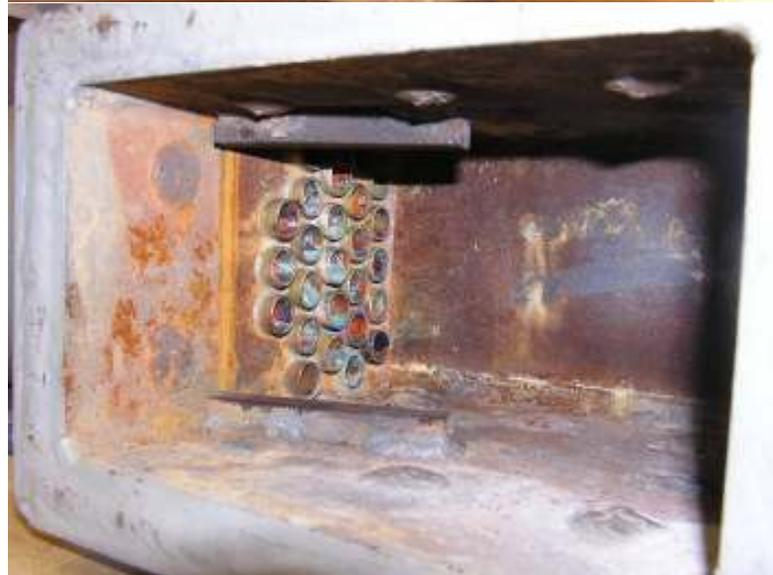
This shows the backhead. The boiler is raised up and with the bottom setting on the cab floor.
