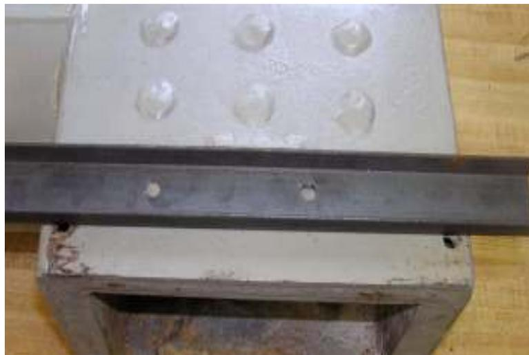
The boiler is ready to be drilled for attachments and plumbing. The plan is to install everything needed to get the locomotive operational and then go back and install the lagging, boiler jacket and cosmetic details.
