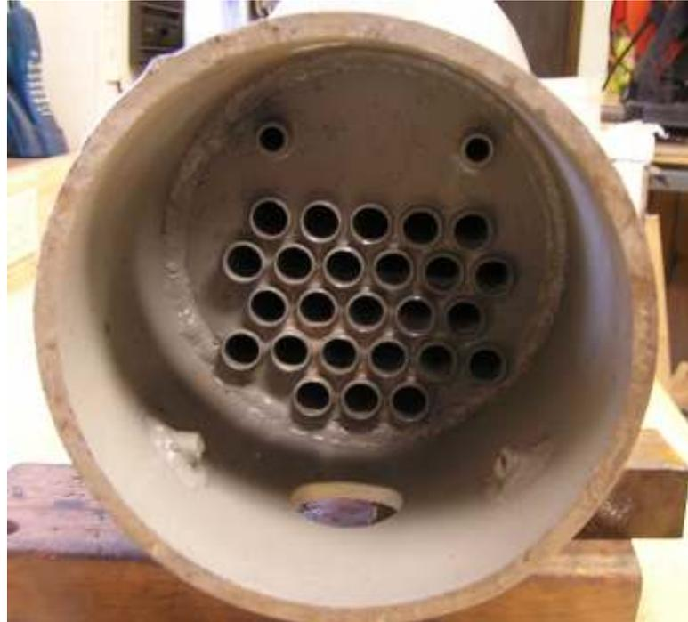
This is the inside of the firebox (the boiler is laying on the right side). The square rods welded to each side of the fire box support a steel plate that goes from the front to about half way back and points up at about a 30 degree angle. The plate is to force the heat to go to the back and then up to the top before dropping down and out through the tubes.
