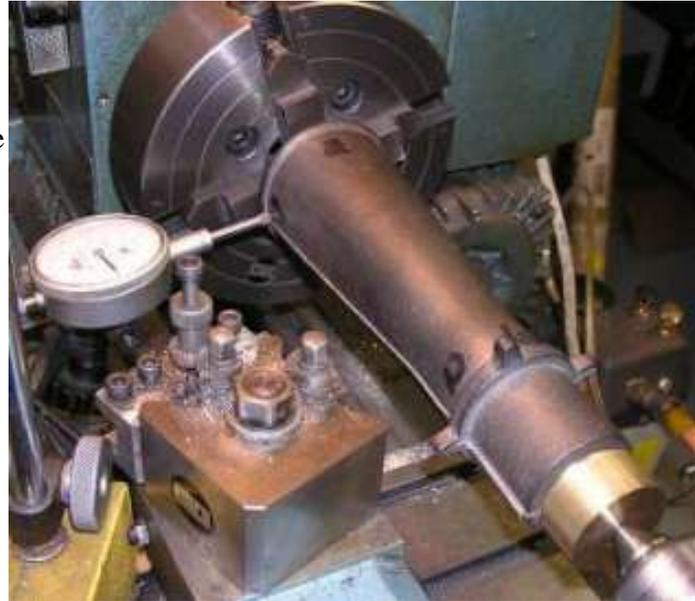
Some voids were found in the base of the smokestack as shown on the right. It almost looks like termite damage. The only area of concern was under the ring and a small area above the ring. Those areas were filled with 550 degree solder and filed smooth ---- almost like lead body work.
