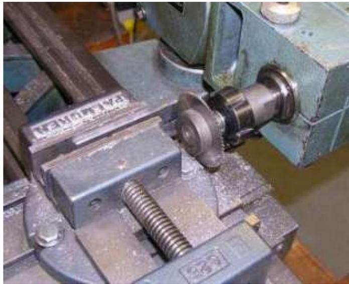
Slots were milled in the cover hinges and the hinges on the door filed to fit. The door was then positioned and retained with the clips and the hinge pin holes drilled through the front and the cover in the same operation.
