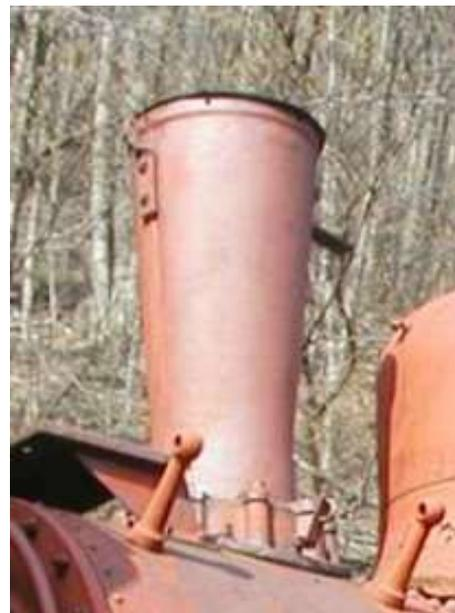
The challenge with the smokestack is to find a way to mount it with the casting centered --- there are no true edges. Also, the lathe doesn't have a steady rest, but not sure how one would work on the rough casting.
