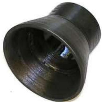
**Smoke Box Front:** Cass 5 front is nearly identical to Kenneth's castings. One difference is that the front is secured with 24 studs rather than the 20 Kenneth specifies.
