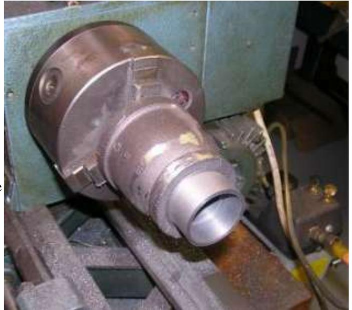
The finished petticoat after an acid bath and shot of WD40. The inside shape is not quite like that shown on Kenneth's drawings. Hope it works.
