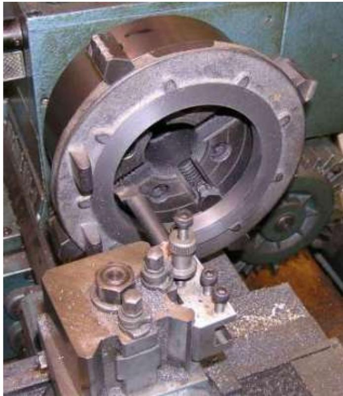
The front was then mounted on the 3-jaw chuck and the outer edge and inside surface finished.
