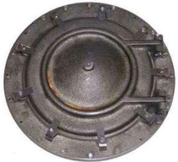
**Blower & Exhaust:** The most difficult part of the blower-exhaust system is the flange that attaches to the bottom of the smoke box. Kenneth suggests that the flange be made from the cutout for the boiler steam dome. I'm having my boiler built by someone else so I didn't have the cutout. A short piece of the 6" schedule 40 pipe was obtained from the local machine shop. The 0.28" thickness seemed excess so I turned the thickness down to about 3/16" I then drilled a
