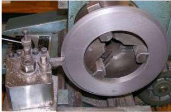
Next, the front was reversed on the chuck, the chuck moved to the rotary table mounted on the mill and the location of all the holes marked with a center drill.
