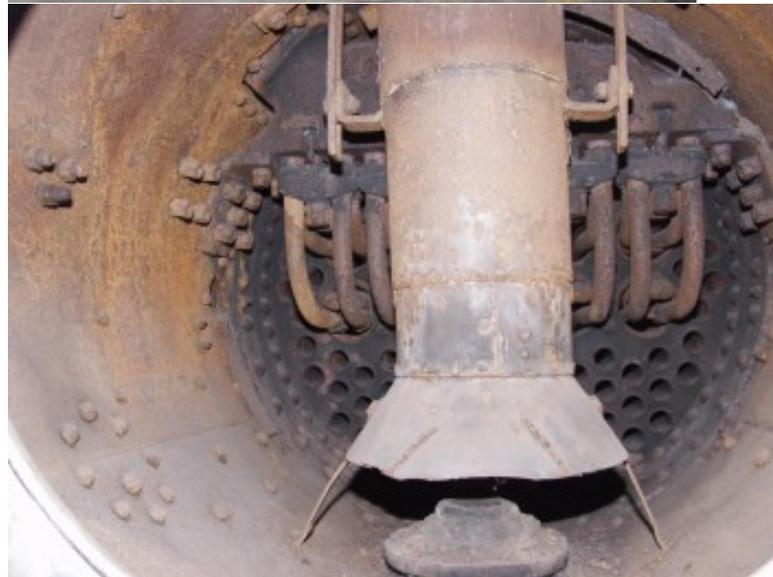
Kenneth suggests steel or brass for the petticoat. The large end is 2.75" diameter and that size brass round bar sells for ~ \$9/inch. Didn't like the thought of boring a huge hole in a big hunk of steel either. So off to the hardware store and came back with the 2" to 1.5" reducer and 1.5" to 1" bushing shown on the right for \$6. Got out the big pipe wrenches and tightened the joint.
