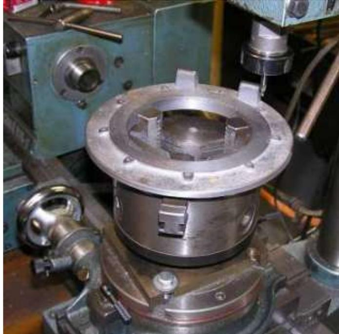
The clips were made from a piece of 1/8" angle. The legs were milled to the correct length and the leg that goes over the door thinned. Each clip was then sliced off with the slitting saw as shown on the right. **(Update 4/15/04:** I was unhappy with these clips --- they were too large and out of scale. I later replaced the clips with cast dogs. There is more information at the end of this page.)
