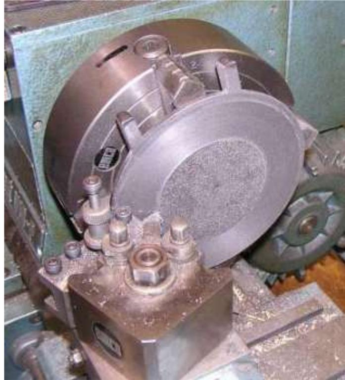
The front casting was mounted and centered on the 4-jaw chuck. The inside was then bored to create a smooth reference. The surface that mates with the door was then skimmed. The little bosses where the clips mount couldn't be skimmed because the tool would hit the hinges.
