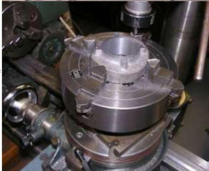
There were two obvious ways to cut that 3.315" radius on the underside; mount it to the lathe faceplate or to use a boring bar/ fly cutter type tool in the mill. Friend Dan Staron said he used a fly cutter.
