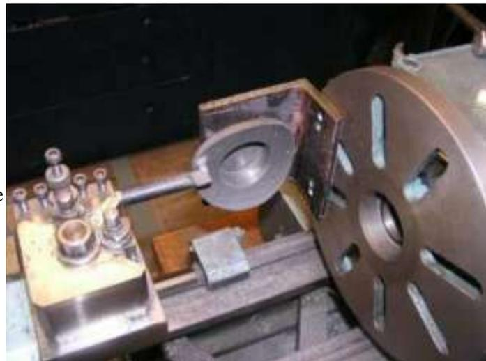
The finish cuts on the lathe went well --- again using low speeds and a fine cuts. The angle and base were light enough and speed slow enough that counterweights were not required.
