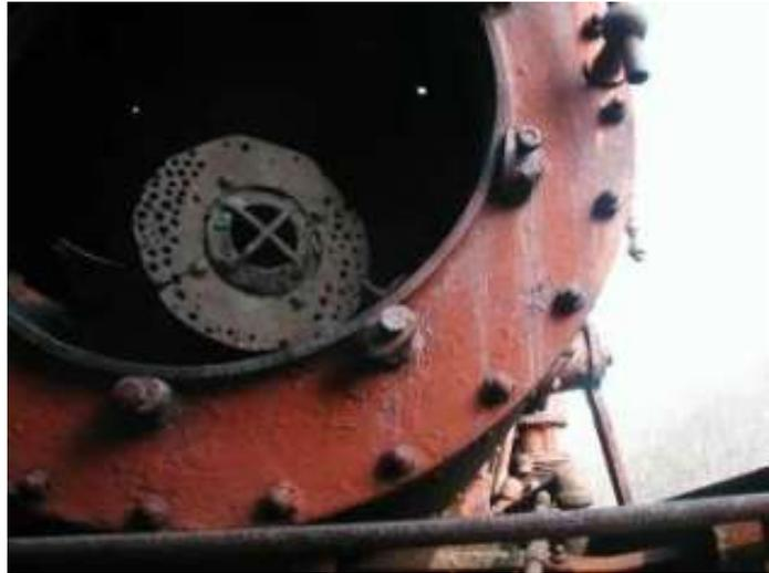
The inside surface of the door must be skimmed so that it will seal. The challenge was to find a way to chuck it in the lathe. The problem was that the steps on the chucks are such that the jaws have to grip the rounded edge of the door casting as shown on the right. Believe it or not, the grip was firm.
