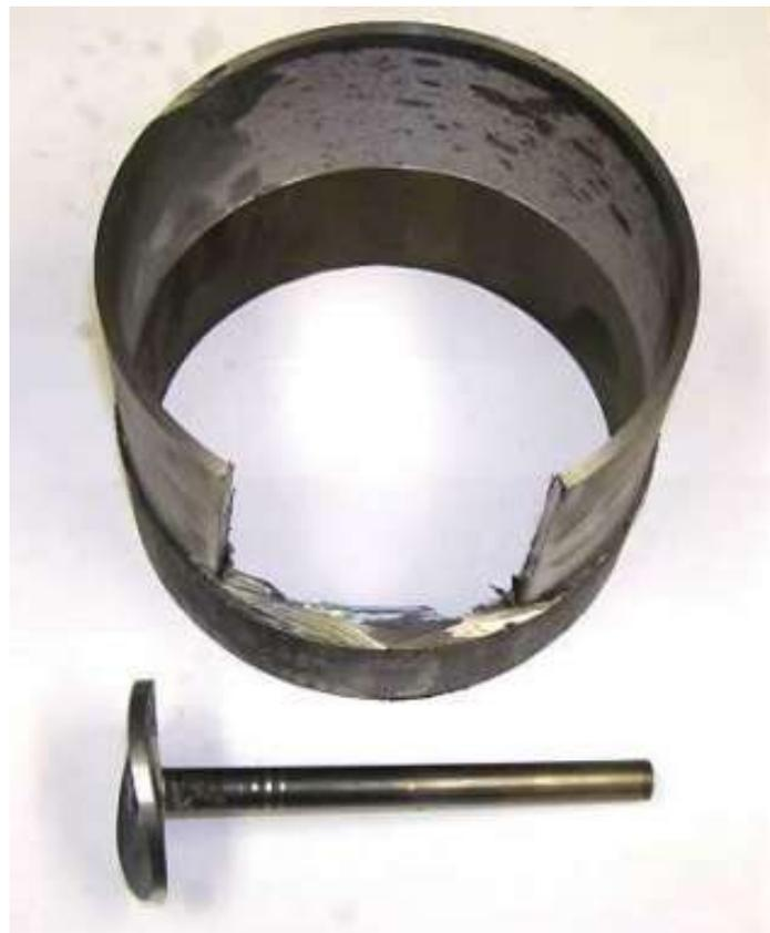
Next, the flange was chucked in the 4-jaw chuck. The end of the rod centered with the tailstock center and the chuck adjusted so that the rod close to the flange was also centered. The chuck was then tightened and the rod cut off next to the flange (hacksaw). The flange was then drilled/bored to ~ 0.975" to match with the OD of a 3/4" copper elbow.
