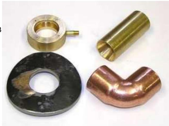
The finished blower and exhaust system after the parts were silver soldered together. The 3/16" nipple is to show the position of the blower input and will be replaced with fittings connecting to the blower line.
