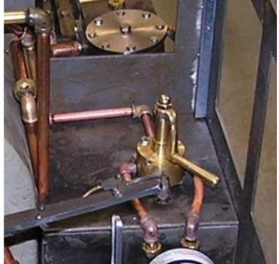
**Brake Pipe Routing:** The pipes run from the valve on the top of the shelf down the shelf front, through notches in the platform top and then bend and go under the frame just behind the firebox to the brake cylinder on the left side. The pipes are identified on the photo on right.
