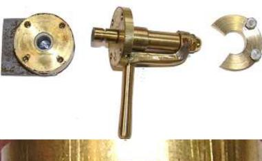
Holes were drilled through each port about 1/32" deep into the plug. The plug was then removed from the body and the slots made between adjacent holes on each side of the plug using a Mototool with cutoff disk and then smoothing with small files. The photo shows one of the slots. There is an identical slot on the other side.
