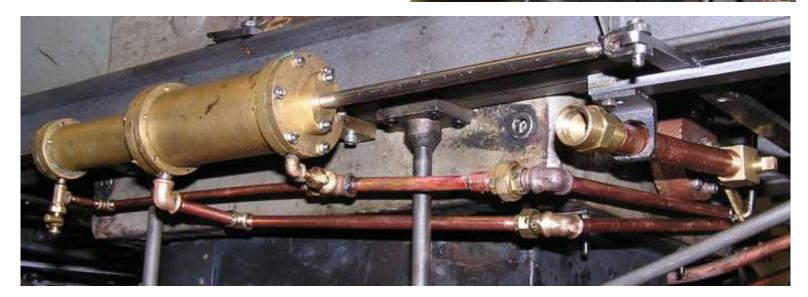
This photo shows the cab interior with the installed brake valve.
