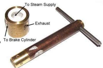
The model worked and made a pretty good seal. Next, a model was made using a 3/4" sleeve OD and a 7/16" plug OD. The valve worked pretty well, leaked slightly at room temperature with 125 psi air applied and leaked only a little in boiling water. The handle was a little hard to turn. Tried another sleeve with a smaller ID to put more pressure on the sleeve and body ---- no difference in force or small leak. Tried yet again with similar results.
