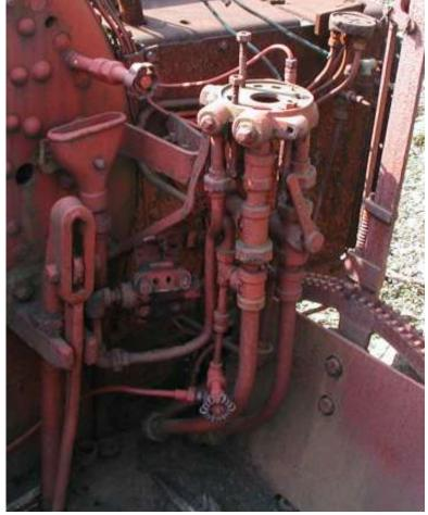
Mike Green also was able to shed light on the air brake mounting bracket. The photo on right taken by Gordon Carlson shows the mounting bracket on Shay #3345, the last narrow gauge shay built by Lima and the one that Mike is modeling.
