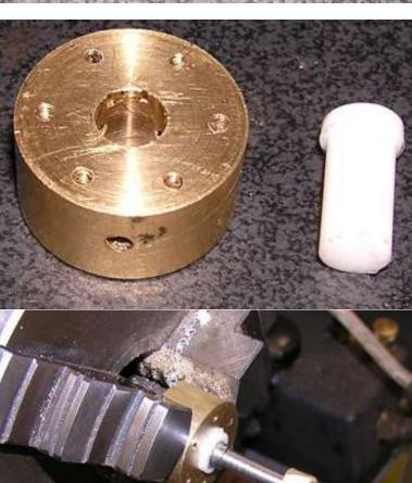
This is the body with sleeve. Note the 1/8" plug in the side hole. The input port below is fitted with a 3/16" MTP nipple and a 1/4" to 3/16" bushing. This was used to test the seal.
