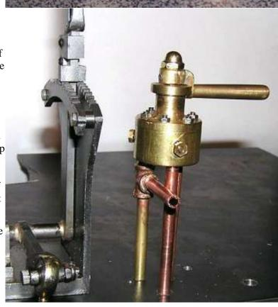
This view is from the left side of the back of the valve. The valve handle is in the **BRAKES ON** position.
