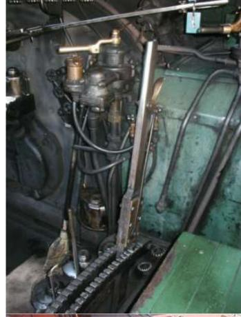
This shows the bases of the two brake valves on Cass 10. Note the pipes below the air brake valve. It's not clear if the valve is supported by the pipes or if there is some sort of support bracket.
