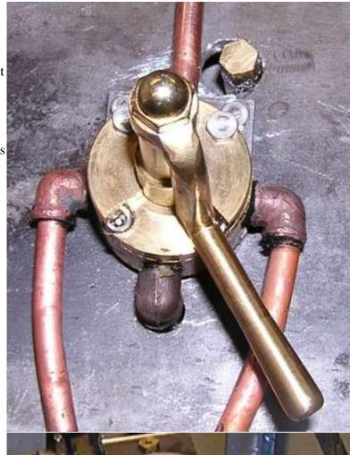
This photo shows the valve mounted on the shelf. The valve is off center to the right side of the shelf to minimize interference with the reverse and throttle levers. The plan is to also mount the whistle valve on the shelf --- to the left of the brake valve.
