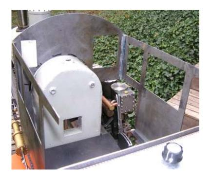
**Update 1/23/04- New Front:** Shortly after I started to install the pipes through the cab front I realized that the window placement was not good. The windows needed to be moved toward the corners by about 3/8" and the lower edge of the windows raised somewhat. I waited until all the pipes were installed and then made the new front pictured on the right. The first front was used as a drilling template for the this second front making the job easy.
