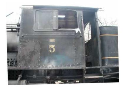
This shows the inside of Cass No 5. Note that the back side of the cab is behind the doors, against the coal bunker. Kenneth's design has the back side in front of the door openings.
