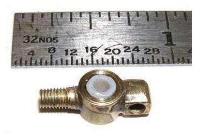
**Plugs:** The plugs were made from 1/8" brass rod. One end was turned down and threaded 2-56 and the other end turned down to 3/32" The only critical dimension is the 0.197" length of the
