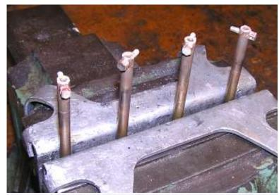
The output port was filed into the final shape at this time. The rod was clamped into a vise to hold everything steady.
