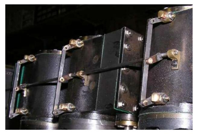
The photo above shows the six cocks mounted in the cylinders. The shaft linking the three cylinders is 3/32" stainless steel. The levers on the shaft are identical to the levers on the cocks. The little bearing blocks are made from 1/8" thick brass and retained by one 2-25 screw per bearing. Note that I've decided not to use the tubes on the discharge side --- at least for now.
