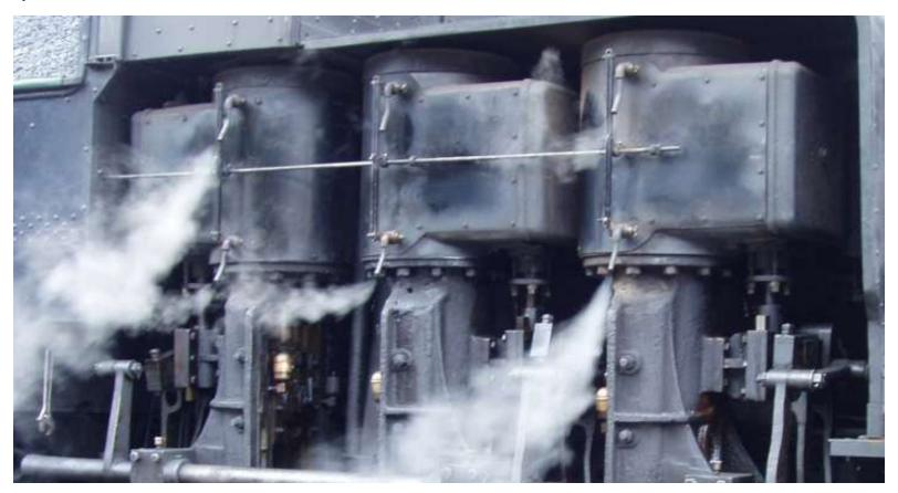
The photo on right shows the cocks on one cylinder in more detail. All 6 are ganged together and operated by a single lever in the cab.
