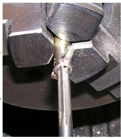
A # 55 drill was run through output port to the input port to make holes through the Teflon sleeve. The sleeve was then reamed 7/64". The photo shows a finished body.
