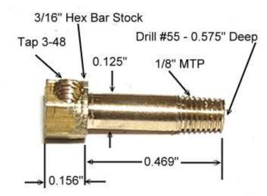
**Body:** The center part of the body was made from 1/4" brass rod. The end of the rod was drilled 1/8" to a depth of about 3/8". The rod was then crossed drilled 1/8" about 1/8" from the end. (The hole in the center of the rod helps center the bit when the cross hole is drilled.) Next, the input/output ports were silver soldered into the rods as shown on the right. Solder was applied around the output port to fill the void between the hex end of the port and the curvature of the 1/4" rod.
