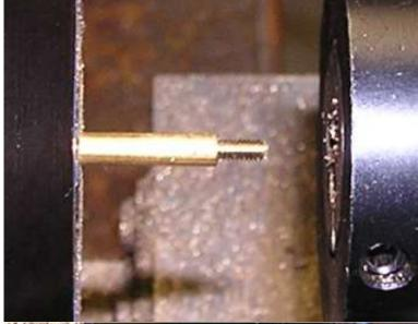
A fixture was made to hold the threaded end of the plug. The lever end of the plug was then turned to 3/32" with the length of the middle section 0.0197" Once the stops were set correctly, it took only a few minutes to turn the ends of 9 plugs.
