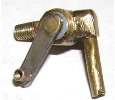
This was my first use of the MTP 1/8-56 die. When I used the die I found the resulting threads too big to thread into elbows. The die as manufactured is not adjustable. I cut a slit in one side using a Dremel cutoff disk and then used it in a die holder where the retaining screws squeeze the die slightly making a smaller OD thread. That fixed the problem. Care was taken when taping the holes in the cylinder to not run the tapered tap in too far making the hole too big.
