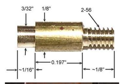
The first step was to turn the end to be threaded and thread with 2-56 die. The rod is held in the lathe collet chuck and the die holder slides on a rod held in the tailstock chuck.
