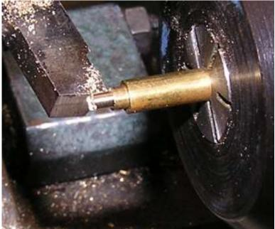
The lever was made from 5/32" wide, 0.050" thick stainless steel. The distance between the holes is 3/8". The plug was soldered into one hole and a brass tube in the other hole. The tube was made from 3/32" rod with the about 1/8" at the end turned down to 5/64" and drilled #49. The photo on right shows the plug just after the soldering.
