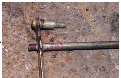
After the 3/32" rod was cut from the handle, the hole in the little tube was tapped 0-80.
