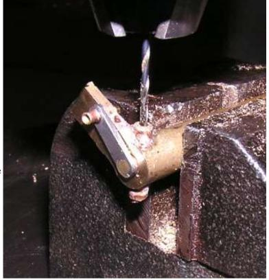
After the hole was drilled through the plug, the burr at each end of the hole was removed by hand turning a 5/64" drill into opening of the hole. The plug was then smoothed with 400 grit Emory cloth (cloth wrapped around plug and held firmly while lever rotated.) This was repeated a half dozen times to get a bright smooth finish. From the looks of plug at the right, it could use some more smoothing.
