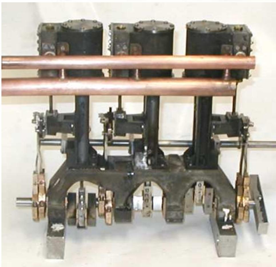
The engine has been operated a couple hours on compressed air and runs very smoothly. It will rotate on as little as 2 or 3 psi pressure. Being an engineer, I was compelled to do a quick power calculation that indicated a power in the 0.5 to 1 HP seems possible. I am now faced with the overwhelming urge to build apparatus to actually measure the power. That should best be postponed till next winter if I'm going to have anything running this summer.
