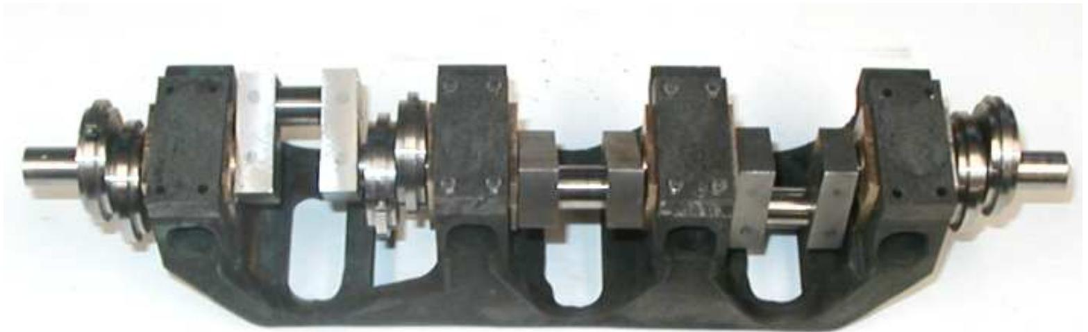
This next photo shows the top view of the lower engine. The aluminum block on the left is a handle to turn the crankshaft. The two larger aluminum blocks hold the engine upright and off the table. These three aluminum blocks are used only for engine assembly and test and will be removed when the engine is mounted to the locomotive frame.
