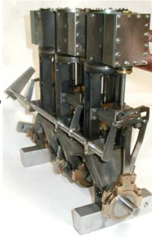
**Side view of engine:** Recall that the Shay engine on the right side of the locomotive. This photo show the outer side of the engine. The rod across the front controls the reversing of the engine. There will a lever attached to the left end of the rod which will in turn connects to a long reversing lever in the cab.
