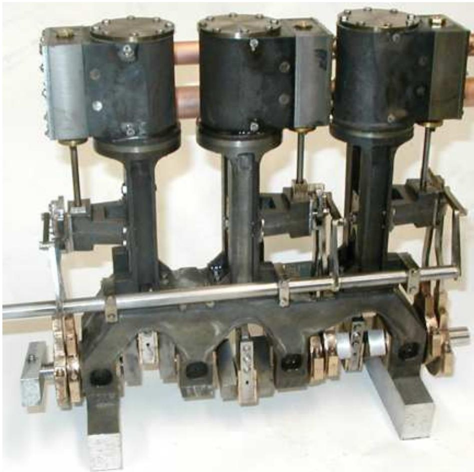
**Rear side of engine:** This is the rear side of the engine that is next to the locomotive frame and boiler. The upper copper pipe is the inlet header. This header has a valve and air line fitting off the photo to the left. These fittings permit engine operation with compressed air. When the engine is mounted to the locomotive this header will be cut near the left most cylinder and a steam supply pipe connected at that point.
