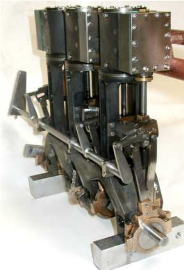
These two photos show the view the front end of the engine. In the left photo the reverse lever is in the position for reverse where the valve for the #1 cylinder is driven by the second eccentric. In the photo on the right the reverse lever is set for the forward direction and the first eccentric drives the #1 cylinder valve.
