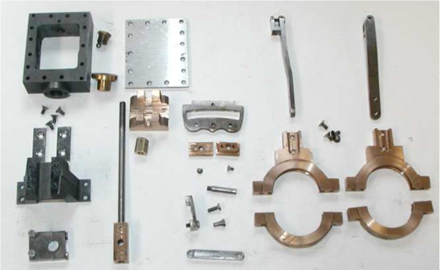
The large bronze parts on the right are the machined eccentric straps. The links blades fabricated from stainless steel stock are shown in the upper right.
