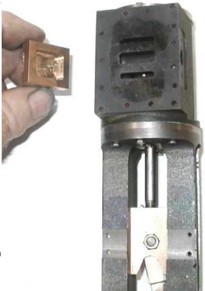
The photo on right shows the cylinder with the steam chest attached and the steam chest cover removed to expose the valve. The upper head is visible as is the snifter valve at the top of the steam chest. The valve stem packing gland is at the bottom of the steam chest. The steam inlet header bolts to the right outside of the steam chest. Steam enters the steam chest from the header via the hole barely visible in the right side of the steam chest.
