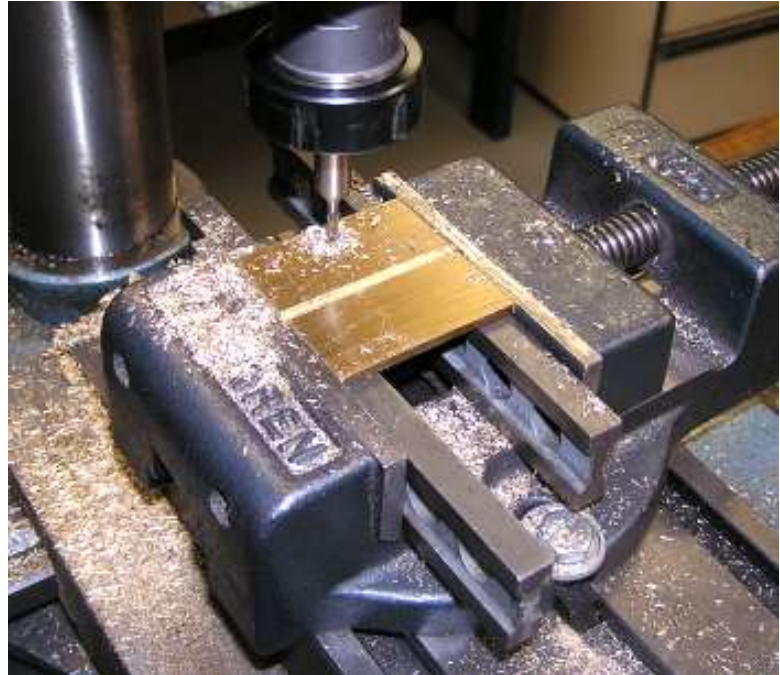
This shows milling the 1/8" wide 1/16" deep slots in one of the ends.
