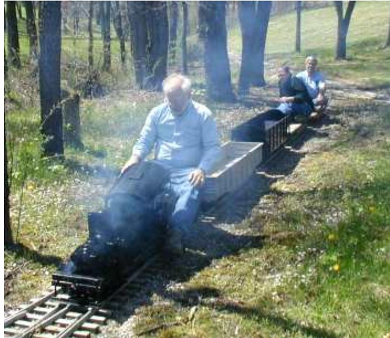
**Lubricator:** The lubricator check valve started leaking and threw oil everywhere as seen in this photo. (The guys said "bet that photo doesn't make it on the website").
