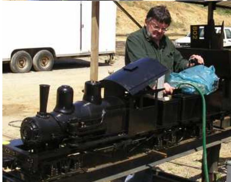
**Building Steam:** The fuel tank was topped off, the air line connected, the atomizer and blower turned on, and the burner lit with a small propane torch. Then it was a 15 minute wait to get steam up. Not sure why I was holding my head ---- maybe I remembered that I promised to mow the lawn.
