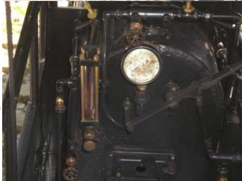
**Repaired Gauge:** Dick McCloy gave me a glass lens to replace the melted plastic one. The gauge was tested later to make sure that it still worked, but it only hissed. This was a \$32 US Gauge sold for use with steam models. A \$10 replacement was ordered from McMaster -Carr. After the new gauge arrived the damaged gauge was opened. The trouble was that the solder
