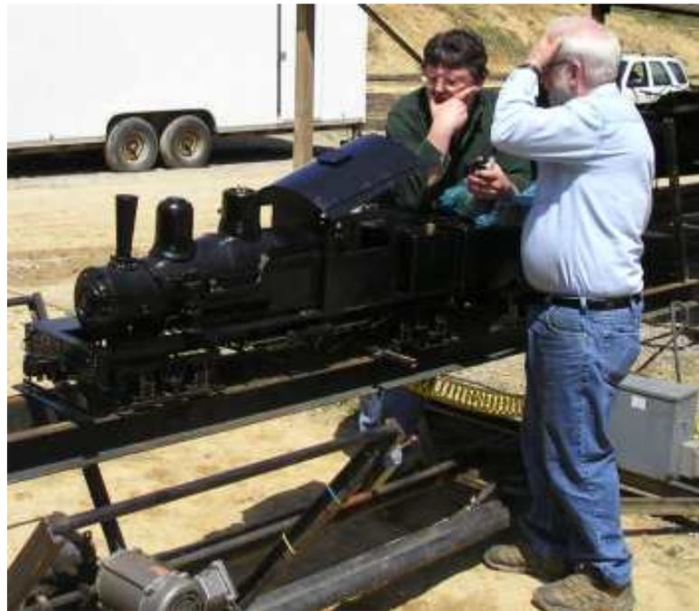
**Steam Is Up:** That's the safety valve going off. I'm switching from air to steam for the atomizer and blower. The air line was then disconnected.
