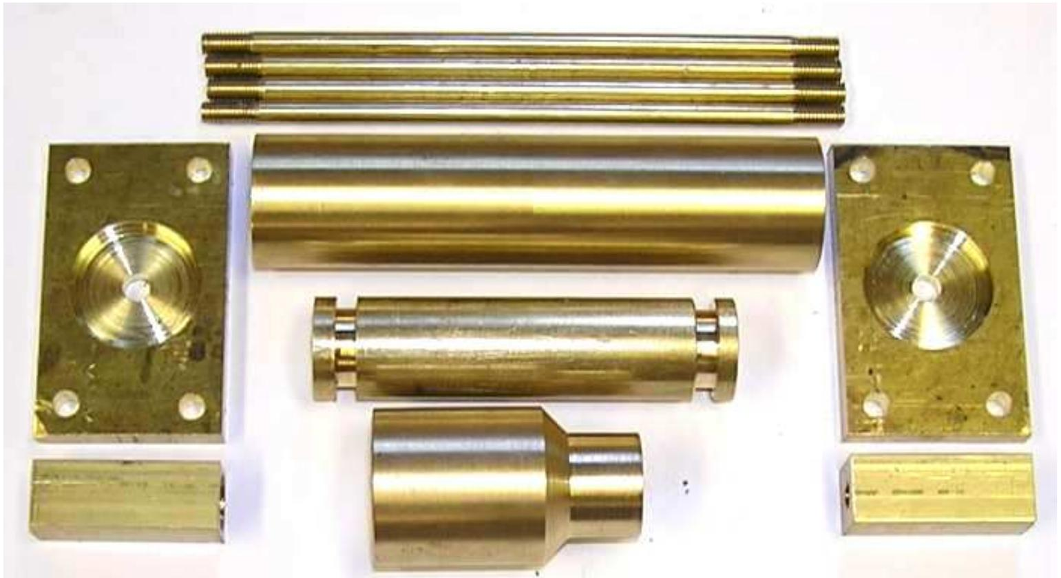
**End Plates:** A 0.025" deep slot was milled in the end plate to match the square piece. This was done so that everything would stay aligned when the two pieces were soldered together.
