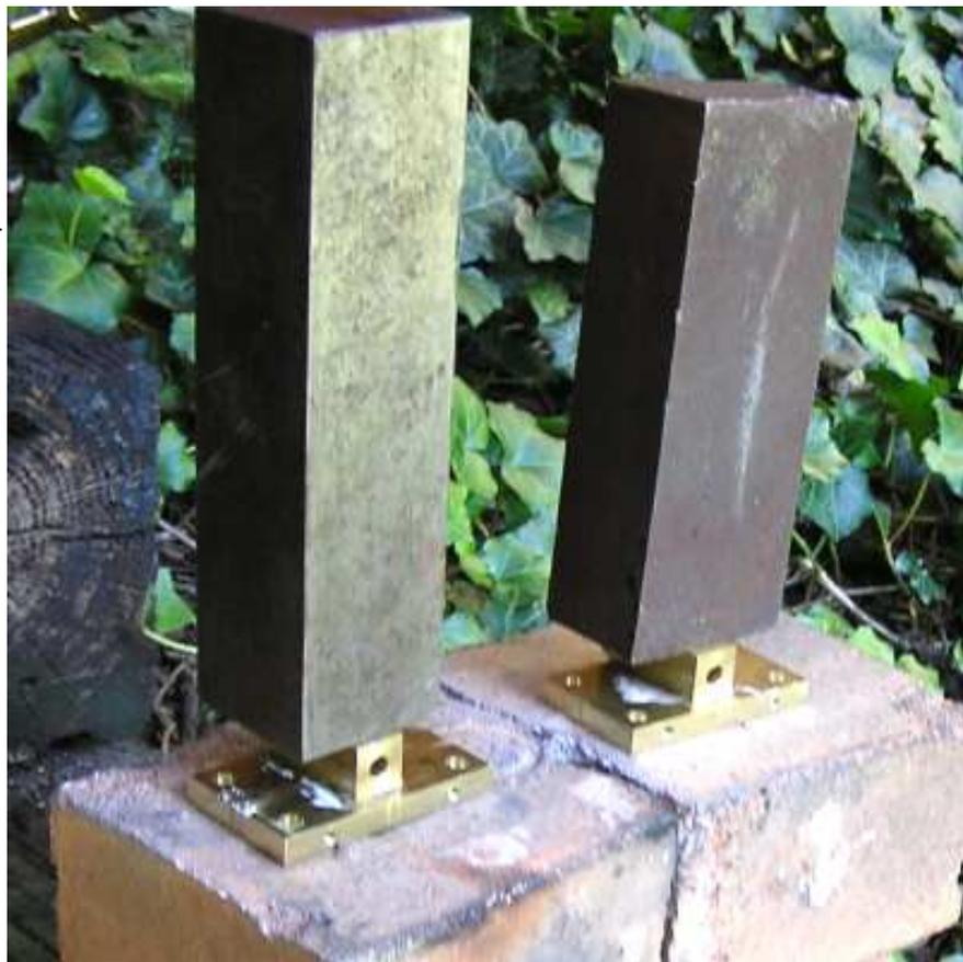
These are the finished end plates. They've been cleaned up some by bead blasting. The flux etches pretty deep so I gave up on cleaning them perfectly. The photo shows the nice silver solder fillet at the joint.
