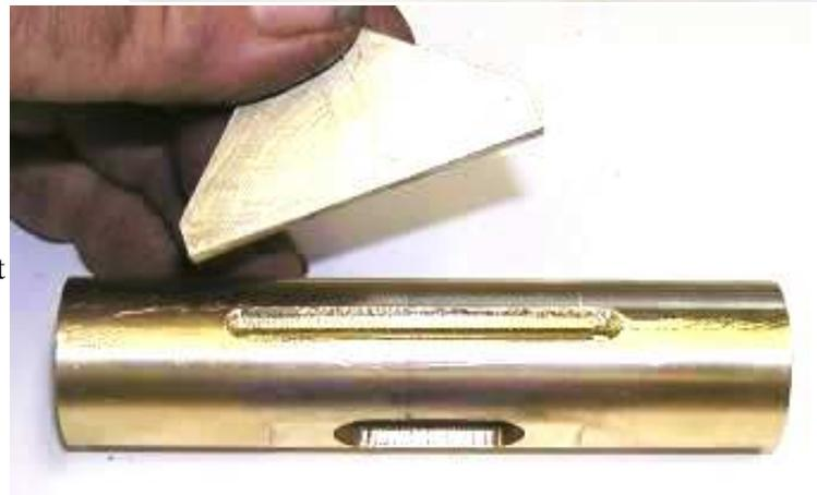
The slot and the bottom of the triangle piece were coated with flux, pieces of flat silver solder were placed in the slot and the plate pressed into position. The pieces were then heated. After the solder flowed the triangle piece was tapped with a hammer to make sure it was seated in the slot. The slot makes a neat way to keep the two pieces in position during the soldering and makes a really strong joint.
