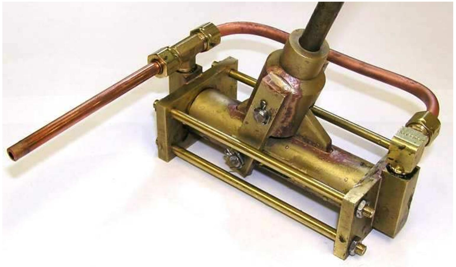
A couple things I forgot to mention. Permatex Form-A-Gasket #2 was used on the pipe threads as suggested by Kenneth. I also used some between the cylinder and ends.
