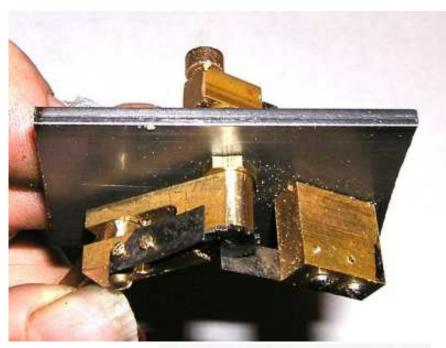
This is the **Ratchet Wheel** and **Shaft** made from the Dremel #199 cutter. The only modifications are that the shaft is cut to the correct length with Dremel cutoff disk (after assembly) and a flat is ground on the shaft for the crank setscrew. Note that the shaft is 1/8" except near the cutter where it is slightly larger.
