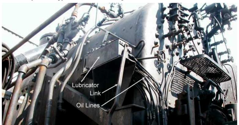
That' a new boiler they're installing. The link connects indirectly to one of the valve eccentrics. As you can see, there are many oil lines. I assume there are many little pumps in the lubricator tank. Next time will have to look more closely.
