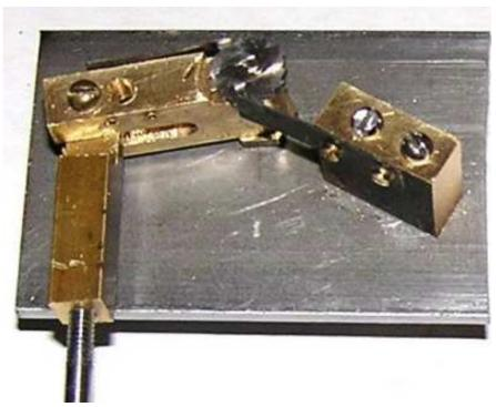
This shot taken from above shows the lever with the lever paw more clearly. The piece on the other side of the simulated tank wall is an early version of the **Crank.**
