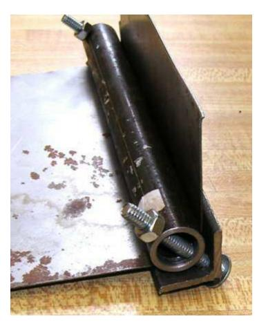
After making a few test bends I realized that the round corners are very forgiving --- the corner can actually be moved slightly if necessary. This capability led me to the basic construction technique ---
