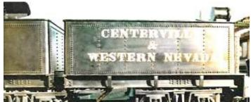
The tender tanks on the Cass shays had been photographed on previous visits in anticipation of building tanks. None of the tanks on the Cass Shays are the same. Also, probably none are original, so one has a lot of latitude here. The tank on Shay No 5 has no rivets, it's welded construction. All of the Cass Shays burn coal so all have coal bunkers instead of fuel tanks.
