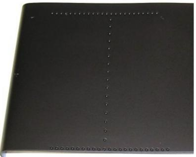
Fuel Tank Construction: I started with the fuel tank. I drilled all the holes in the rear end piece first as shown on the right. (The piece is actually square, the distortion is due to camera angle.) After confirming that the hole pattern was correct, I used this plate as a pattern to drill an identical hole pattern in the front and rear end pieces for the water tank.
