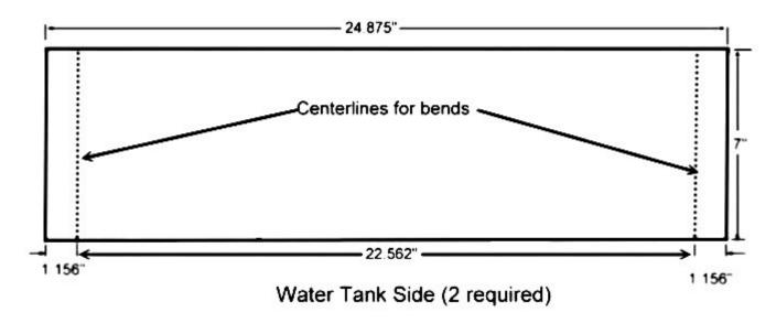
**Sheet Metal List:** After all these computations I was able to make up the material list for the steel store. Kenneth had suggested 22 gauge for the sides and bottom and 16 gauge for the top. I decided to use galvanized steel and make things a bit heavier: 20 gauge for the sides and ends and 14 gauge for the top and bottom. The complete list is:
