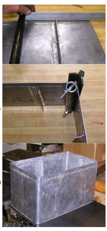
This is the rear side, Still have a lot of rivets to install. Before proceeding I smoothed all sharp edges with a file. Shay Tanks Part I Page 10 of 12
