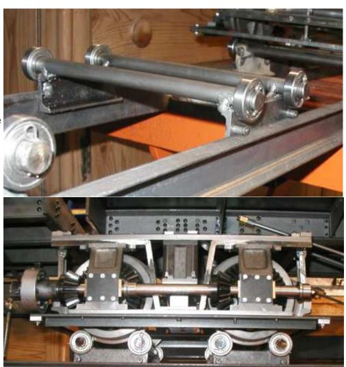
This photo shows a pair of fixtures under the middle truck. (The line shaft is only partially complete at this point.) The wheels turn very freely. This will allow me to spin the wheels and go no place ---- which is the objective.
