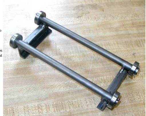
There are 1/4" pins welded into holes in the channels to hold the channels above the rails as shown on the right. The fixture can be used on the Transporter as well as on regular track. The fixture can also be set on a flat workbench. However, the truck would be free to pivot so I'm not sure that would work very well.
