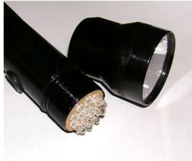
The LED unit was then pried out of the end of the body. At this point it was determined that the LEDs are wired in parallel on the little printed circuit. Two wires go from the printed circuit to the switch area.
