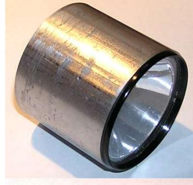
The back was rough cut from 1/8" steel and then turned on a mandrel to the correct OD. The back will be soldered in place later.
