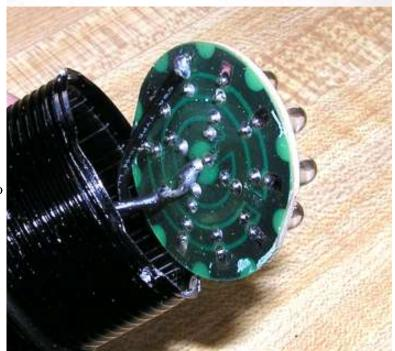
The flashlight body was sawed in half just behind the switch to access the wires at the switch. Note the resistor; it's 2.7 ohms. The resister serves to limit the current to the LEDs.
