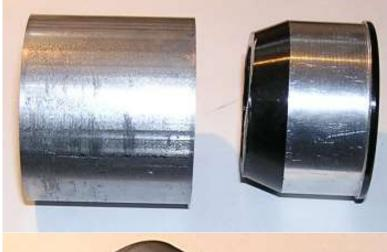
This shows the lens piece inserted in the case. It's a nice fit. A screw through the bottom of the case into the lens piece will be used to secure the lens piece.
