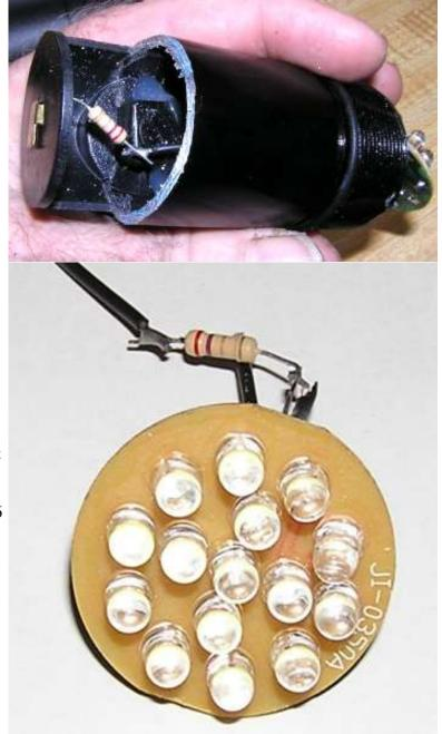
The equivalent resistance of the resistor plus diodes at 4.5 volts input is (4.5 volts divided by 0.4 amperes) about 11 ohms. Similarly, the equivalent resistance at 3.6 volts input is about 18 ohms.
