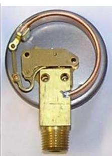
**Utility Gauge from MSC:** This gauge is listed in the catalog as a Utility gauge with no brand name. The catalog says it has a bronze tube and brass movement and a max temperature of 160 degrees F. The accuracy is listed at +or- 5% of full scale at mid scale. This is MSC part # 65303695. The box indicated it is made in China. The lens turned out to be glass, not plastic. Price \$5.01
