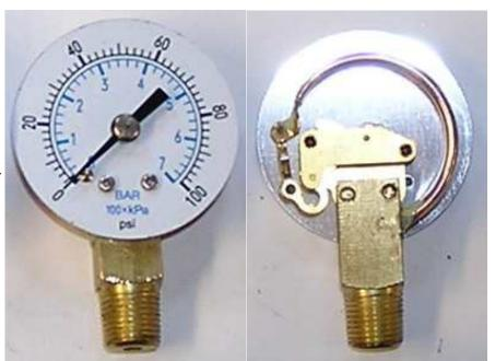
Ashcroft Gauge from McMaster: This is McMaster-Carr part number 3846K1. The catalog lists it as Grade B accuracy (+or- 2% of full scale at mid scale) with bronze tube, polycarbonate (plastic) lens and a max temperature of 150 degrees F. The little gear is plastic. This gauge appears to be made in USA. Price \$9.92
