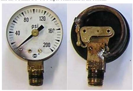
US Gauge from MSC: This is the Ametek Series 500 gauge. The gauge box lists it as Ametek, U.S. Gauge division, made in China. The MSC catalog lists it as Bronze tube with Grade B accuracy (+or- 2% of full scale at mid scale). This is MSC part # 65303695. The lens is polycarbonate (plastic). The construction is nearly identical to the gauge above. Price \$4.33
