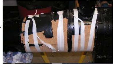
This photo shows the middle section after the second layer of cork was applied and the adhesive set. Note that the front jacket section is in position.
