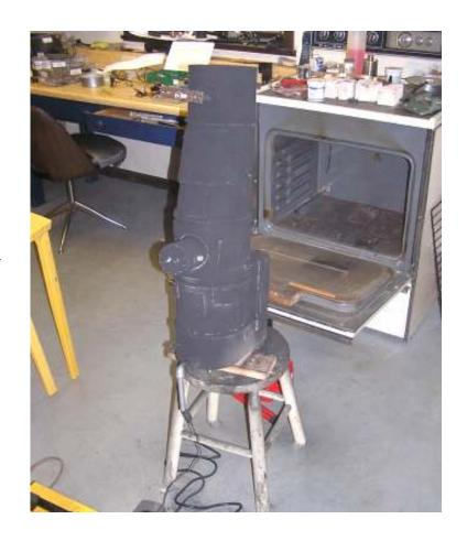
After the front end and under side were powdered with the boiler upright, it was turned to the normal horizontal position with the smoke box end on the oven door. The powder was then sprayed on the back part of the boiler and the backhead. This photo shows the boiler after some more powder was sprayed and the boiler slid part way into the oven. Note the thin areas on the rear side of the jacket spacers. More powder was sprayed so that everything was covered.
