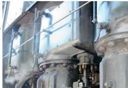
Cass 5 Cab Interior: The following are some photos of the interior of Cass No 5 (80 ton Class C built in 1905). This gives some idea of the plumbing on the real thing. This first photo shows the right side of cab with two brake valves (one steam, one air) and throttle. The unit at top of boiler with 5 valves on the bottom I think is a lubricator --- of the displacement type I assume. That's the long throttle lever above the two brake valves.
