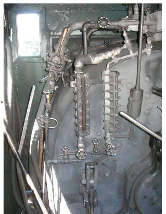
This is the left side of the boiler with a good view of the dual water gauges. I think that's the injector just to the left of the boiler.
