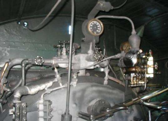
This is the steam manifold on the top of the boiler. A good view of the boiler end of the throttle and the top of the two water gauges on the left.
