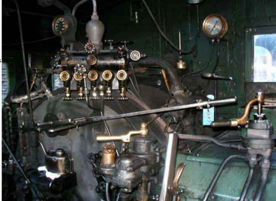
This shows the lower right side with a good view of the reversing lever. Several different types of oil cans are required plus a pretty good supply can. Also note that the interior of the cab is painted green.
