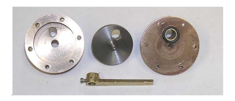
The photo on right shows the back of the assembled valve with 1/8" NPT stub that will screw into the boiler.
