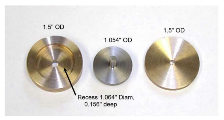
The photos above and on the right show the three main pieces. The outer disks are turned from bronze --- left over from making crankshaft bearings. Brass or stainless would also work great. The middle disk is stainless steel. The next step was to drill and tap six 4-40 holes on a 1.25" bolt circle to hold the two bronze pieces together. The holes in the thinner piece were threaded.
