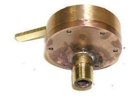
The front of the finished valve. The operating lever is retained with a 2-56 screw. Two orthogonal holes were drilled in the shaft so the handle can be mounted on either side.
