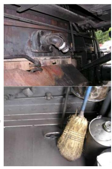
This photo shows the blowdown valve operating handle beside the broom. The handle is lifted to open the valve. This is also Cass No 5.
