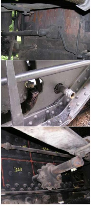
The blowdown valve I decided to make is like one that Jim Buchanan (Buchanan Machine Works) uses on his Climax. Jim sent me a copy of the design from May/June 1997 Live Steam. Jim later told me that he would not use this design again because scale eventually builds in the boiler and the scale then cuts the O Ring necessitating frequent replacement. He suggests a design with bronze body and stainless type wiper. Since
