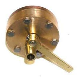
**Update** (12/07/03): The blowdown valve was installed in the back of the boiler as shown in the next photo. A short piece of 5/16" stainless drilled to 15/64" was silver soldered between the blowdown and the elbow in the discharge path. This was after a 5/16" MTP brass nipple broke. This stainless tube has an ID very close to 1/8" pipe so there will not be much flow restriction. A 3/8" OD soft copper tube threaded 1/8" NPT on each
